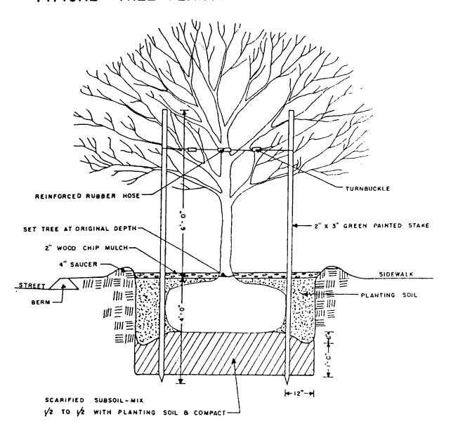
NOTE: GUYING SYSTEMS EMPLOYING BUCKLES & CABLE, SHALL BE BROUGHT TO TENSION & TURNBUCKLE THREADS BE FLATTENED TO PREVENT LOOSENING.
