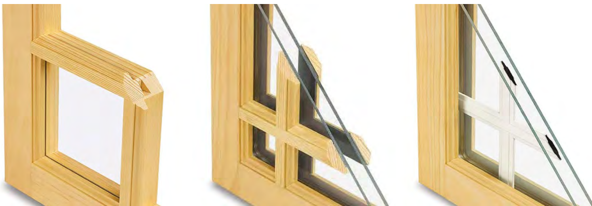
Muntin of a true divided light with insulating glass in a replacement window (left), exterior false muntin (center), and interior false muntin (right). True divided lights are encouraged, though their muntins can be thick compared to what would have been present in a historic window sash due to the thickness of the insulating glass. Decision would have to be made as to the visual appropriateness of a thick muntin in the context in which it is to be used. An exterior false muntin of appropriate thickness is acceptable. Interior false muntins are discouraged because of their poor visual appearance. (Images: Marvin Windows)
