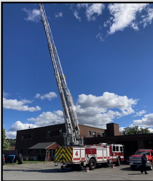
NFPA Ladder Testing on Ladder 4
